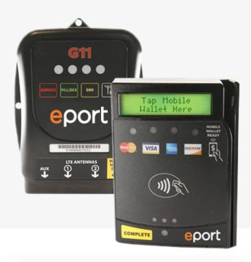
The G11 Cashless Kit allows retailers to accept digital payment options — including EMV contactless, magstripe, NFC card payments, and mobile wallets — and securely capture the critical transaction data required to improve machine performance and boost sales.
