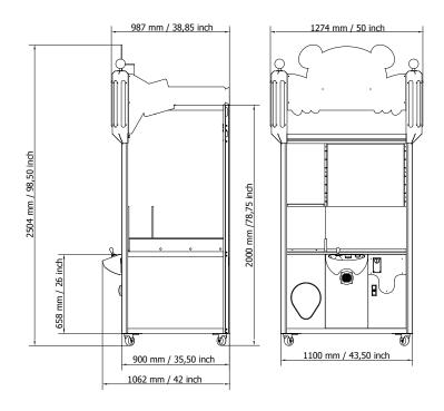
Weight: 225 kg / 496 lbs Voltage: 230V / 115V (50/60 Hz) Power: 125W (typ) / 210 W (max)
