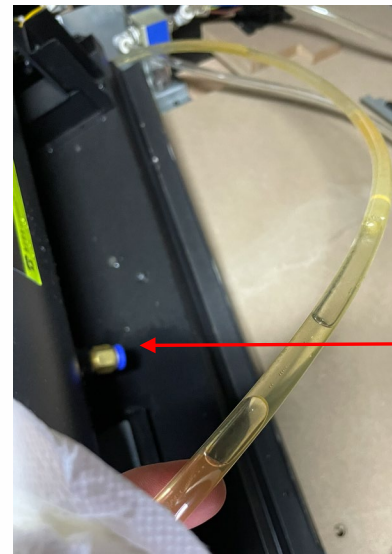
Compressor Drain plug
